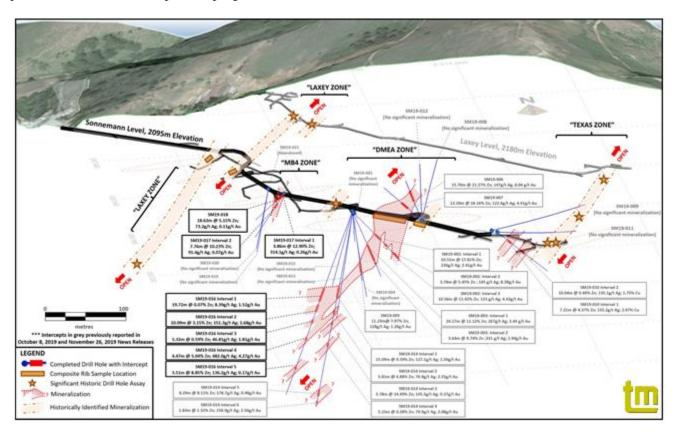
**Figure 1:** 3D Perspective View inclined at 20 degrees looking north-north-east, showing locations of rib-sampling, priority target zones, and the phase 1 drill holes and highlighted the recent SM19-016, SM19-017 and SM19-018
